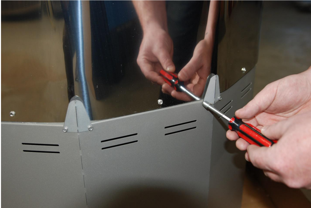
Figure 12 – Removing Base Brackets
