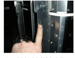
Locate the hole in the back left chamber hinge.
