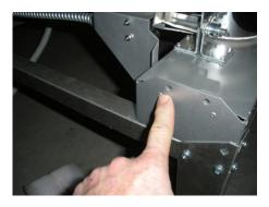
Locate the 2 holes in the right left floor base. Of these 2 holes, you will be placing the other end of the spring into the inner most as indicated.
