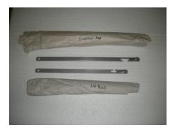
Locate the included Chamber Safety and Lid Support Bars. You will note, as indicated in the image above, that the Chamber Safety Bar is the longer than the Lid Support Bar. Pay attention to the notched portion at the end of each bar. These notches will face the back of the kiln when installed.
