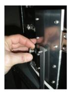
Thread the "T" nut onto the stud. The collar on the T nut will fit into the hole of the chamber safety bar and should be threaded on entirely. Tighten with pliers or wrench.
