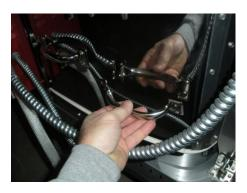
The handle located on the back right of the kiln chamber must be removed for proper operation of the lid support bar. We do recommend that the screws be placed back into the holes to cover any sharp edges.
