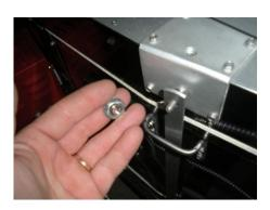
Thread the "T" nut onto the stud. The collar on the T nut will fit into the hole of the lid support bar and should be threaded on entirely. Tighten with pliers or wrench.
