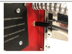
Plug the power interrupt plug into the power interrupt jack.
