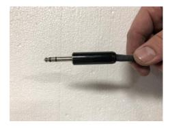
Locate the power interrupt switch cable plug.
