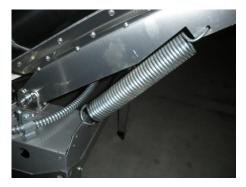
Properly placed lift assist springs, back right. When installed the right side assist spring will look as shown.
