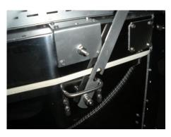
Place the lid support bar through the wireform catch as shown.
