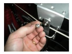
Thread the acorn nut on to the stud and tighten with pliers or wrench.
