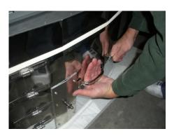
Grasp the kiln chamber as shown: hands towards the rear of kiln should be facing up and hands towards the front of kiln should face down. This hand orientation will make rotating and controlling the kiln chamber easier if the chamber needs to be rotated to navigate narrow doors or hallways.
