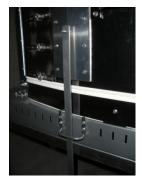
Place the chamber safety bar through the wireform catch and onto the mounting plate stud as shown.
