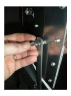
Thread the acorn nut on to the stud and tighten with pliers or wrench.
