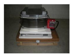
Remove the shipping container cardboard outer "tube" and packing material from around the kiln.
