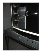
You will note a mounting plate with stud on the left side of the kiln chamber. You will also notice a wireformed catch directly below it. These items are involved with the installation of the Chamber Safety Bar.
