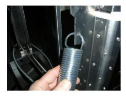
Insert the end of one spring, from the inside of the hole as shown.
