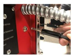
Locate the power interrupt jack located on the rear of the main control enclosure.
