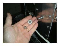
Remove the acorn nut and "T" nut from the kiln chamber mounting plate.
