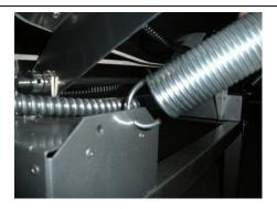
Have one person rotate the chamber up from the front chamber handle. (The chamber should be held there until all 2 lift assist springs are attached).
