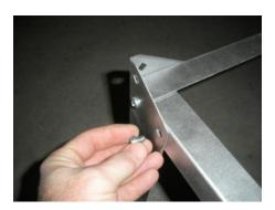
Locate the 2 long metal piece and 2 short metal pieces removed from the container previously. Along with the 4 angled top stand legs these will form the kiln stand.
