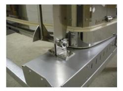
Place the chamber hinge ears in between each of the floor base hinge ears as shown. The floor base hinge ears are angled and slotted which allows for an automatically alignment and fit. The kiln chamber is now properly placed.
