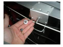
You will note a mounting plate with stud on the right side of the kiln lid. You will also notice a wireformed catch directly below it. These items are involved with the installation of the Lid Support Bar. Remove the acorn and T nuts.
