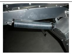
Properly placed lift assist springs, back left. When installed the right side assist spring will look as shown.
