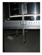
Installation of the chamber safety bar is now complete. Now would be a good time to double-check that the notch on the chamber safety bar is facing towards the back of the kiln as shown. If it doesn't look like the image above, remove and remount properly.
