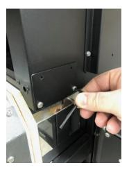
Once the brackets are removed. Rotate them so there are two holes facing the stainless jacket on the existing kiln. Do so with all 4 mounting brackets. Refer to Image.
