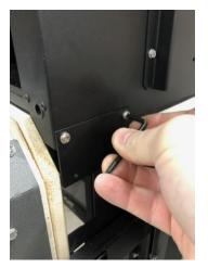
To mount securely, attach the LT mounting brackets to the existing kiln using the included #6 1/2" Hex Head Screws. Mounting of the LT will require you to drill through the stainless jacket on your existing oven. We do recommend using an all or small punch to create an indentation in the metal jacket to allow the screw to bite into the metal. Repeat on all 4 corners.
