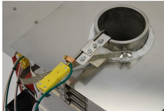
Immersion Thermocouple placed within the salt pot and held with mount
