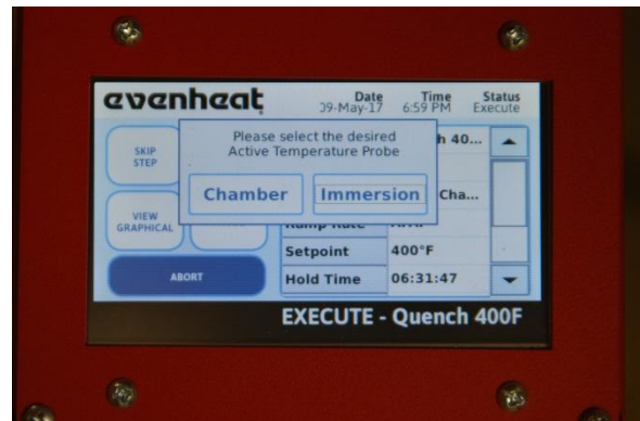
A dialogue box appears, press “Immersion” to select the Immersion Thermocouple. The dialogue box disappears and you are now controlling from the Immersion thermocouple.
