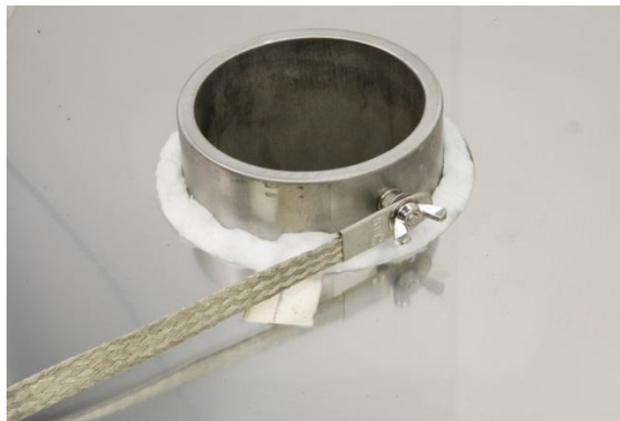
Salt Pot Ground Strap Attached to the Salt Pot
