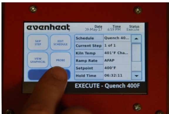
Press the "PROBE" key to select Active Thermocouple
