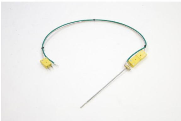
Chamber thermocouple assemblies properly assembled.
