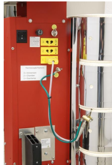
Over-Temp Thermocouple Properly Installed
