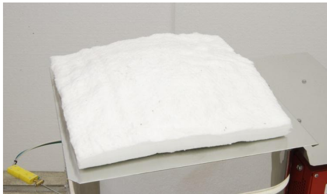
Refractory Fiber Placed over the Salt Pot Replacement Part #06423.300
